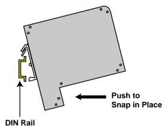
Gently push the chassis toward the rail to snap it in place. A "click" sound verifies that the attachment is secure.
