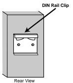
To mount the chassis, hook it onto the DIN rail with the top of the clip, as shown below. The chassis will hang down.
